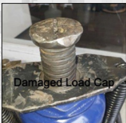
Damaged load cap typically flattened edges or score marks across load surfaces
