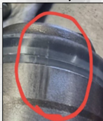
Scored Piston & Seal assembly
