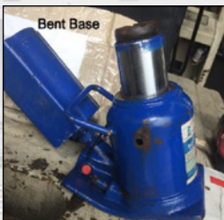
Bent Jack base typically bent at corners
