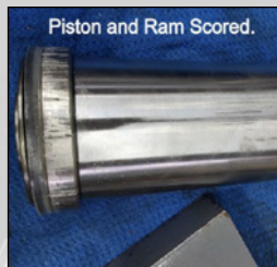
Scored Piston & Seal assembly
