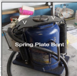
Dent top of reservoir of damaged return spring saddle
