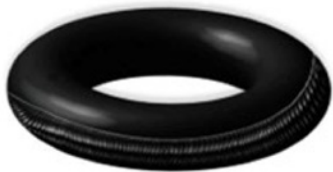
Scored Barrel Damage
