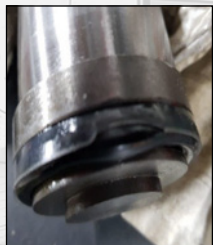
Seal damage & gouged barrel
