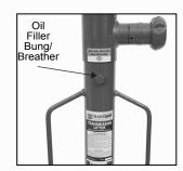
3. With the pump pedal in the raised position turn the release valve knob anticlockwise one complete turn (Lock Open).
