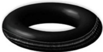
Scored Barrel Damage
