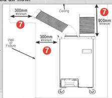
3 Installation of Extended Hot Exhaust Ducting to Outdoors – (Optional) Hot Exhaust discharge air can be removed from the airconditioned space with flexible duct.
