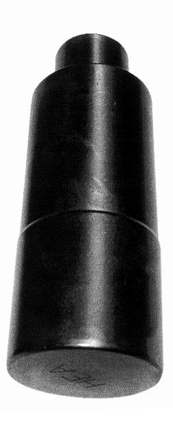
Different size bushes for assembly and removal of bearings and bushes.
