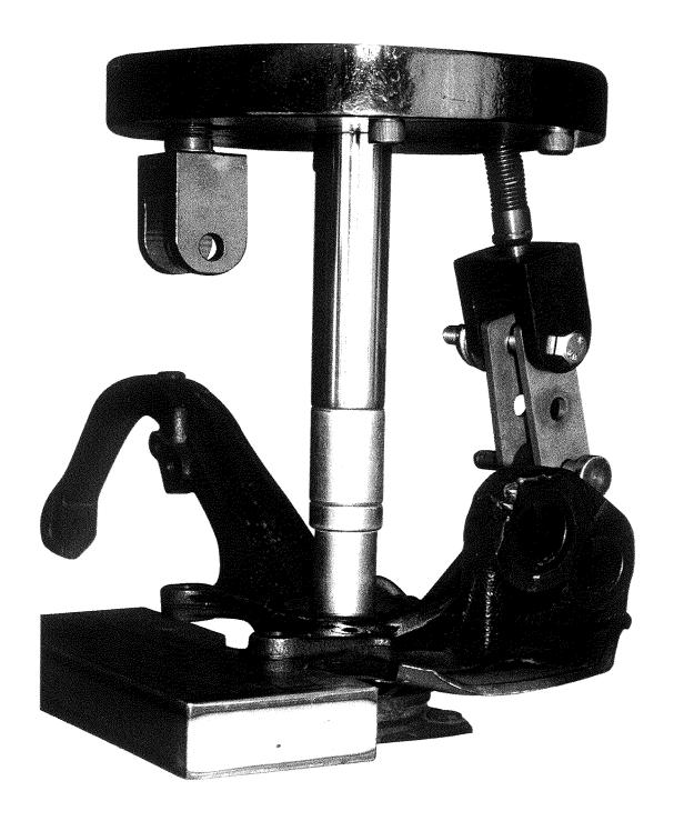
Removal and assembly of bearings. Common tool.
